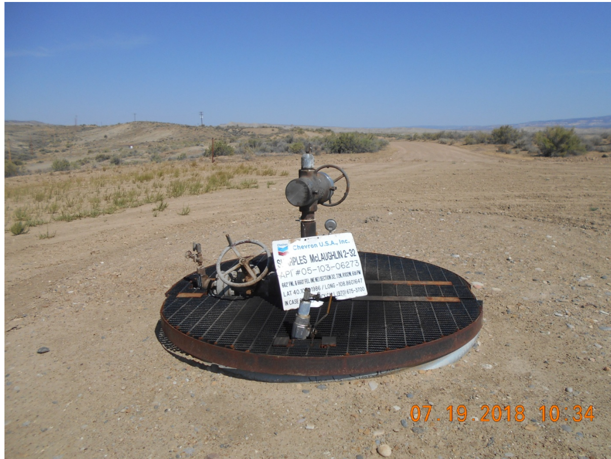
Injection Wellhead
