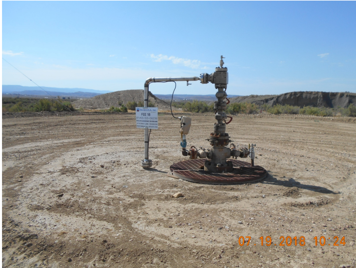
Injection Wellhead
