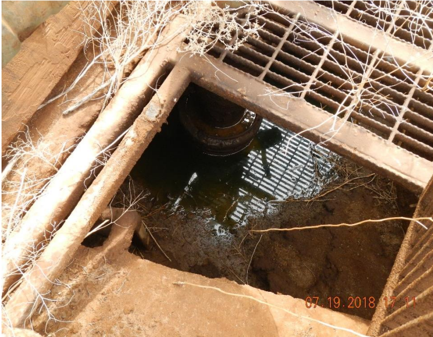
Fluid level in well head cellar.
