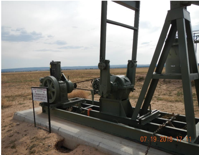
Taylor #3 pump jack with chain attached to prime mover.
