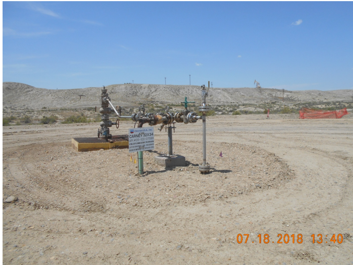
Injection Wellhead
