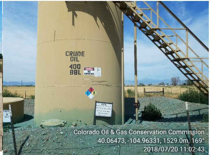
Photo 2. Tank battery
