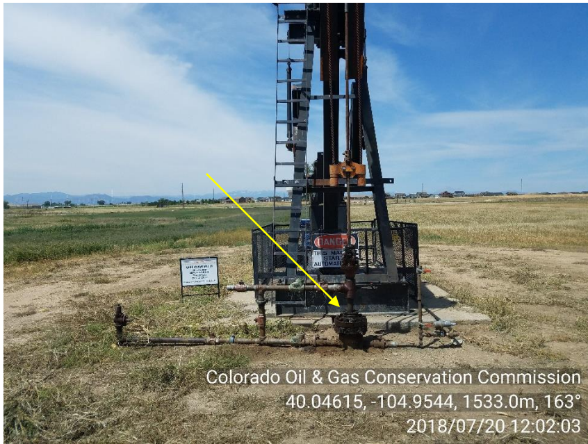
Photo 1. Wellhead/ stuffing box leak/stained soil
