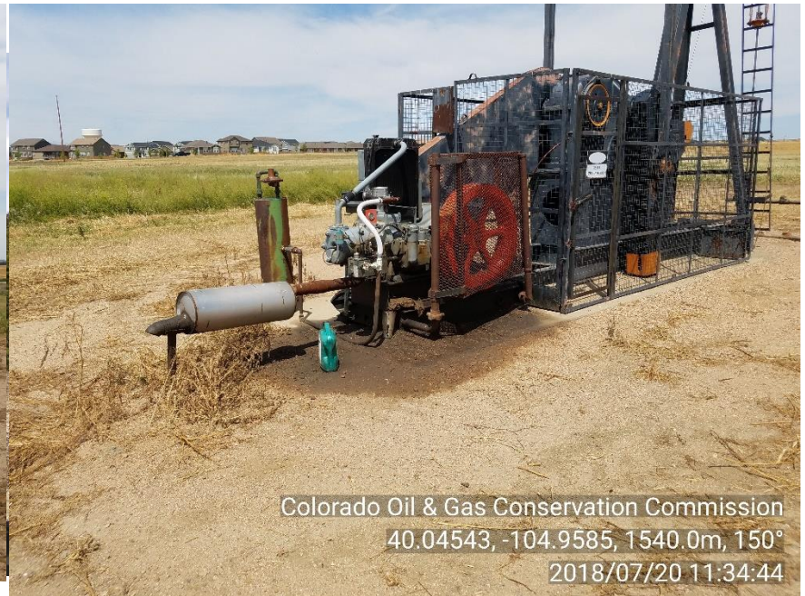
Photo 2. Stained soil near pump jack prime mover
