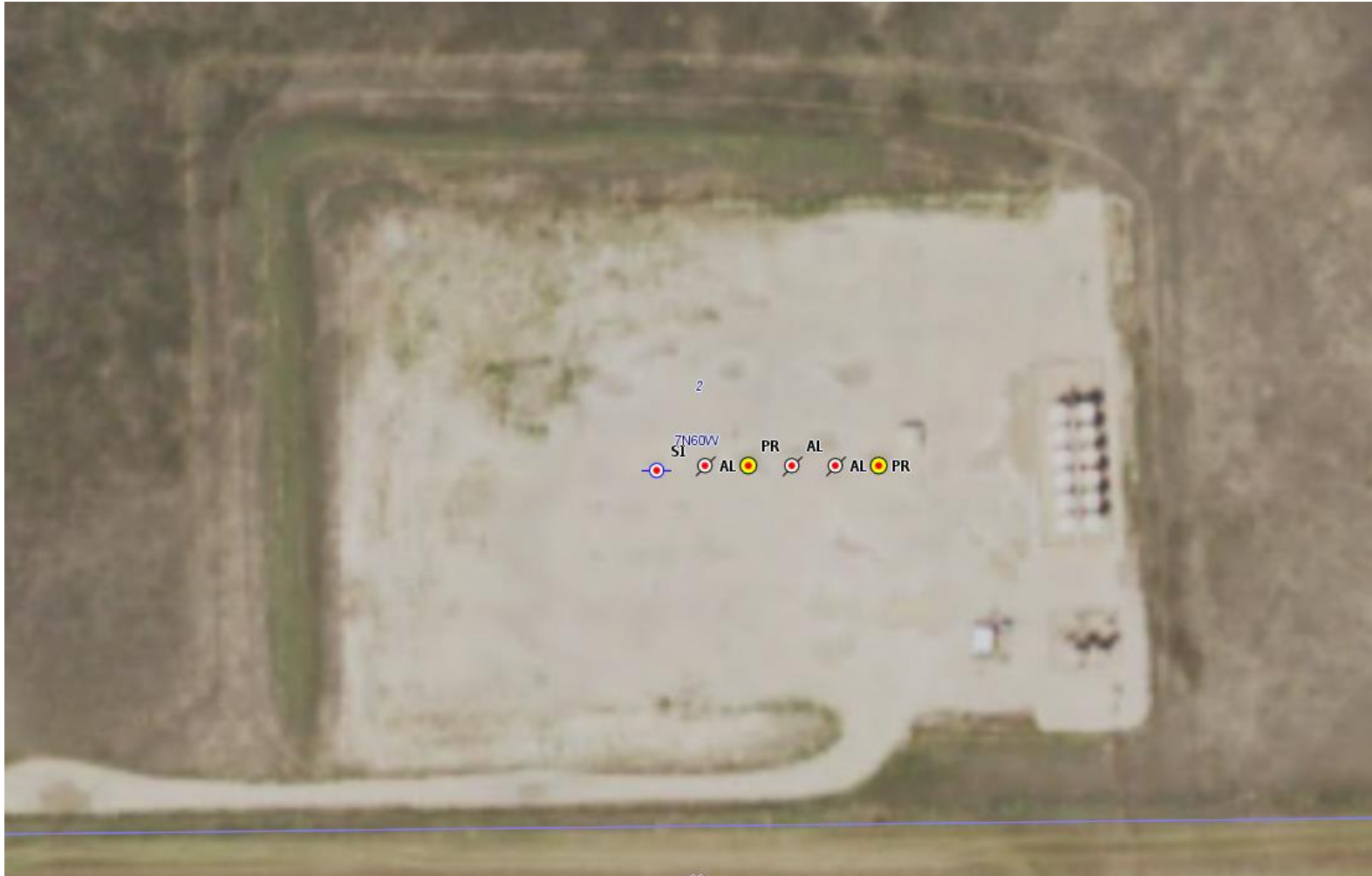
Photo 17: 2017 COGIS aerial imagery. Photo shows areas on the west end of the location that do not appear to be necessary for production operations. These areas need to be reclaimed in accordance to COGCC 1003 interim reclamation requirements.
