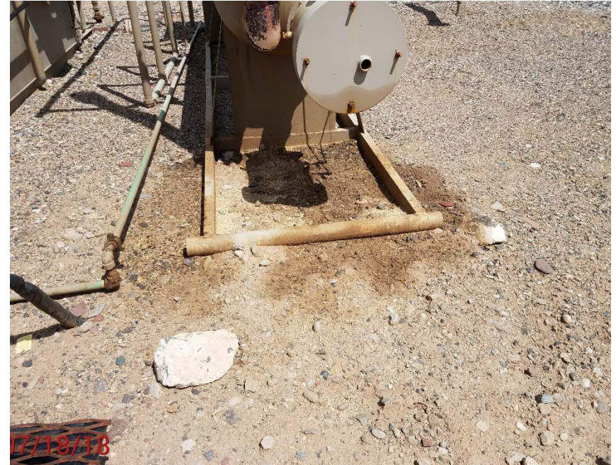
Location Photo #4, Stained ground under low stage vessel
