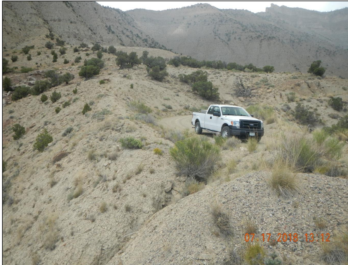
Erosion of hillside from ditch run off and rilling of roadside @ (39.48523 108.04113)
