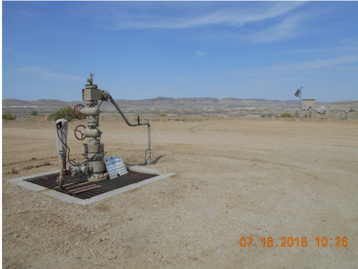
Injection Wellhead
