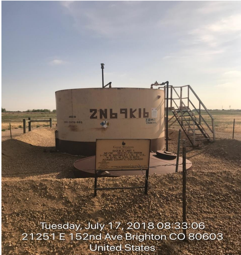
Photo#1 Production tank and produced water pit
