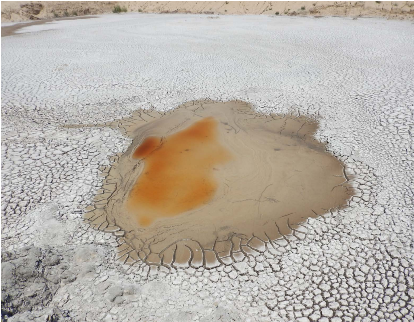
4 ft by 6 ft area of oil observed on pit.
