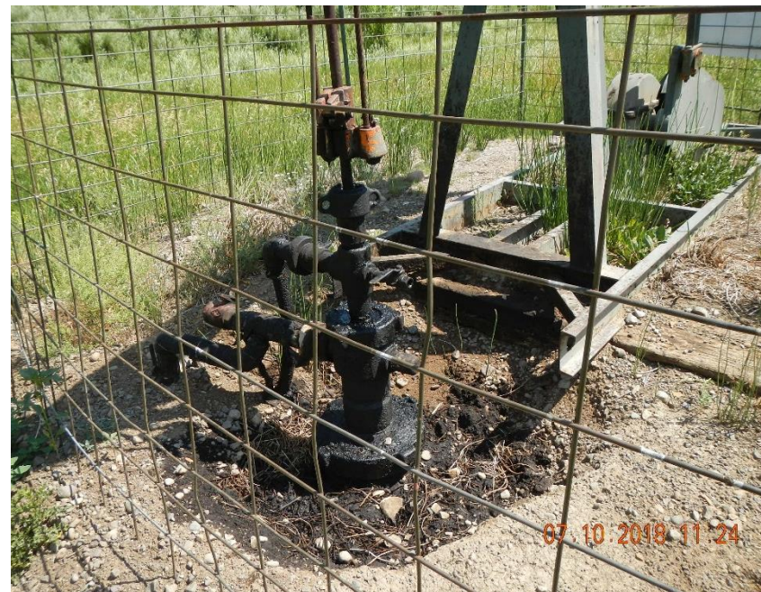
Well head is wet and surrounding soil is stained with oil.
