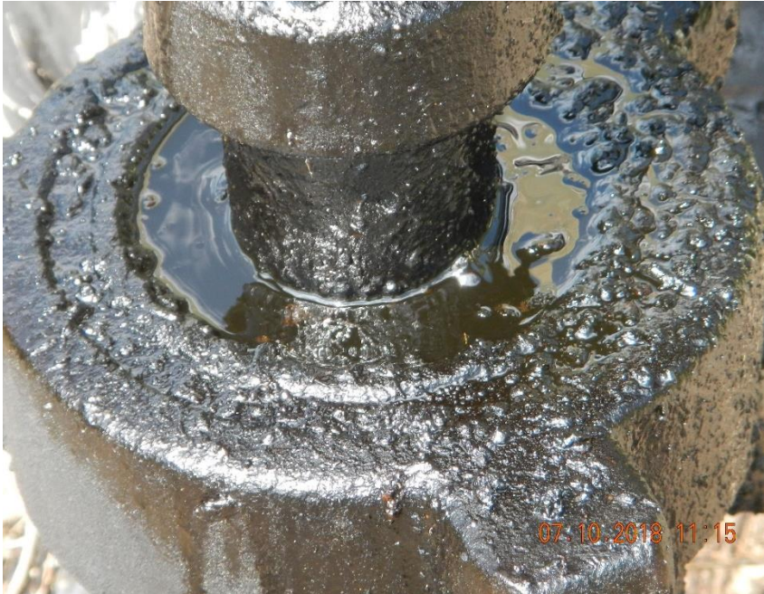
Gas bubbling out of oil on well head.
