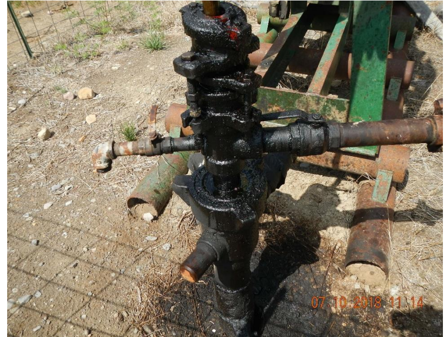
Well head is wet and surrounding soil is stained with oil.
