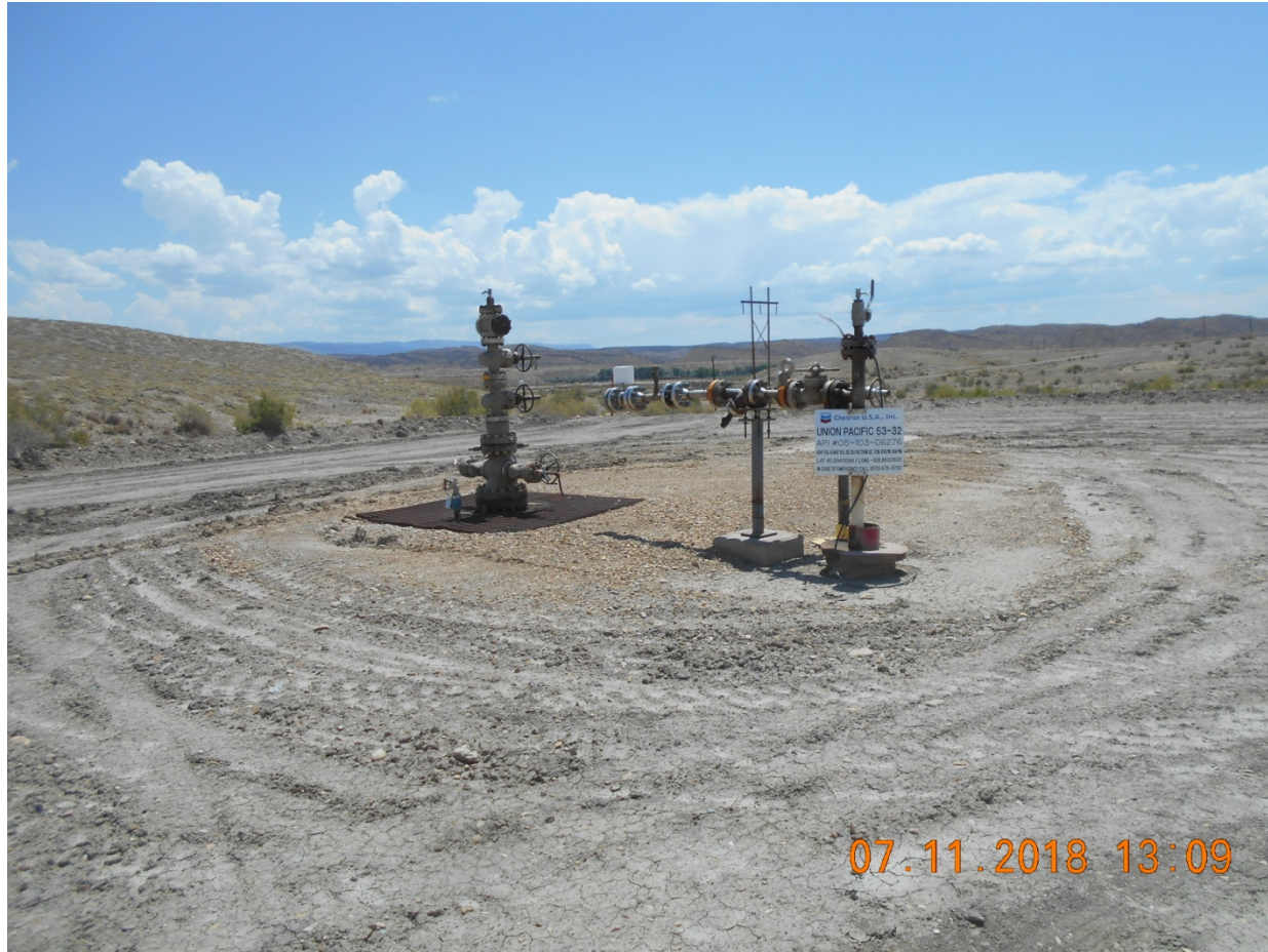
Injection Wellhead
