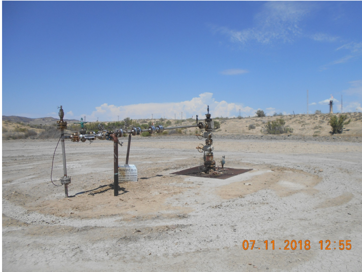
Injection Wellhead
