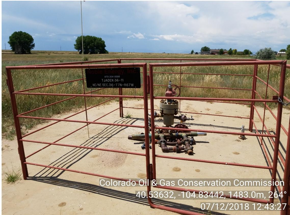
**Wellhead. Corrective Action: Remove trash/unused equipment to comply with 603.f**
