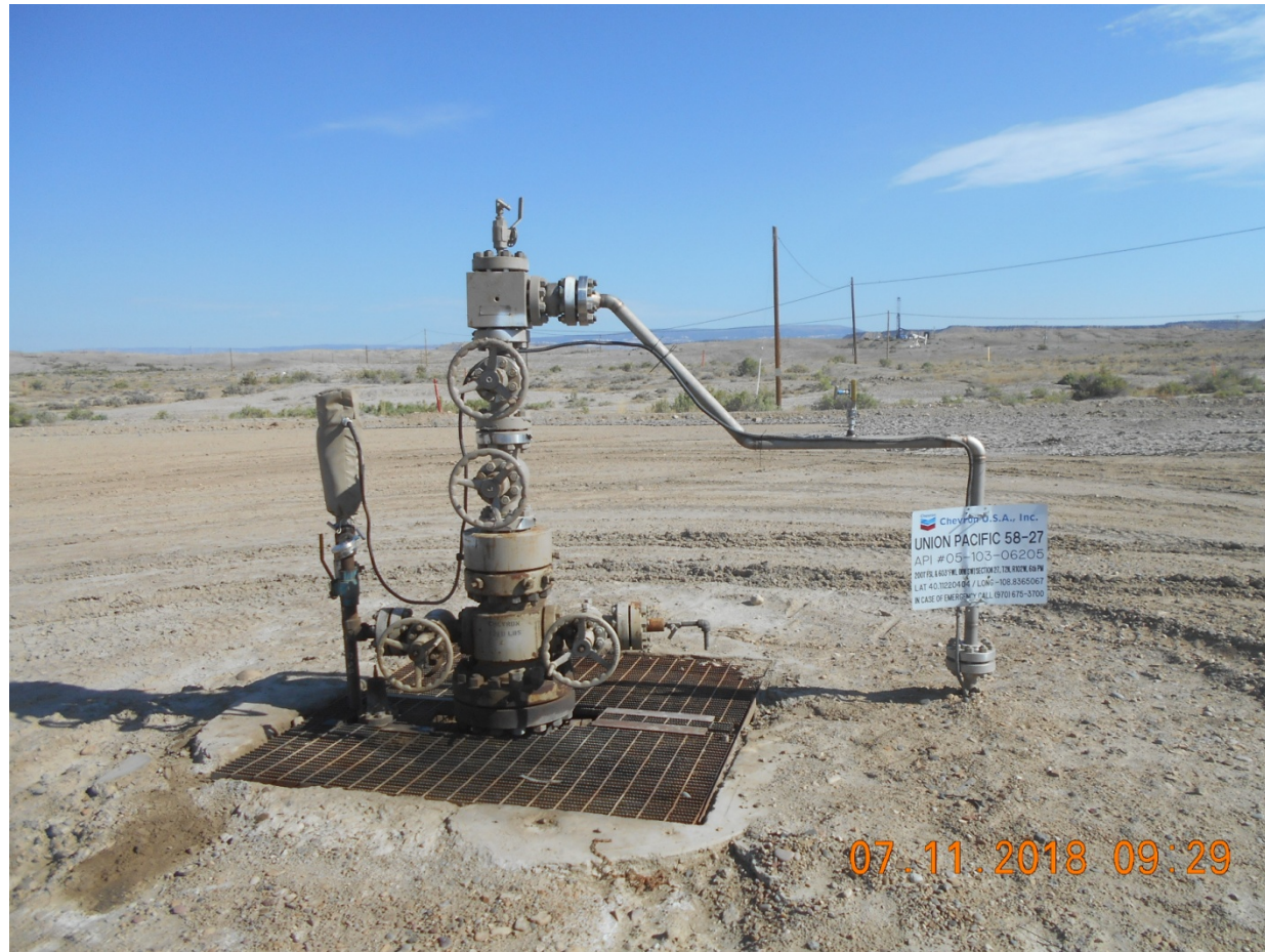
Injection Wellhead
