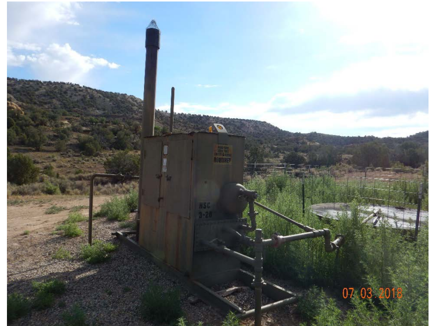
Photo #4 – Operator was notified of an audible leak detected at heated horizontal separator on inspection date.
