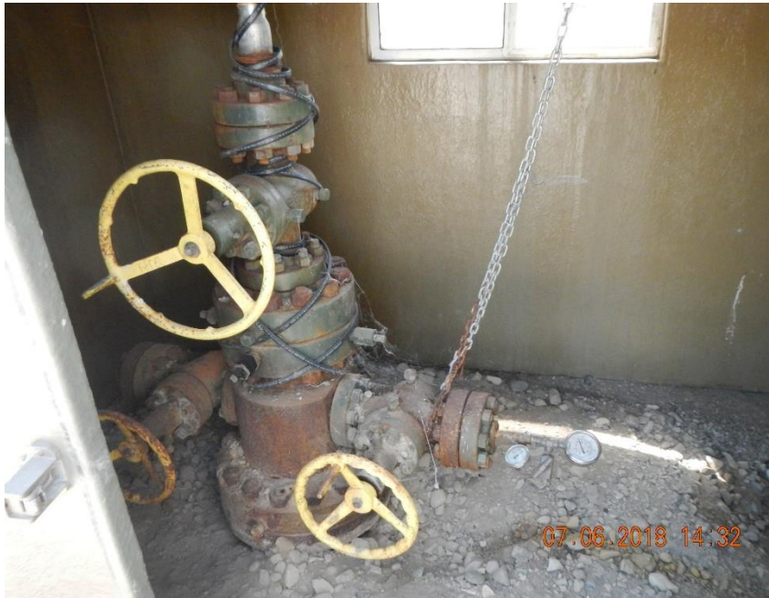
Tierra Piedra 33-5 #15-1 SWD well head within fiberglass shack.
