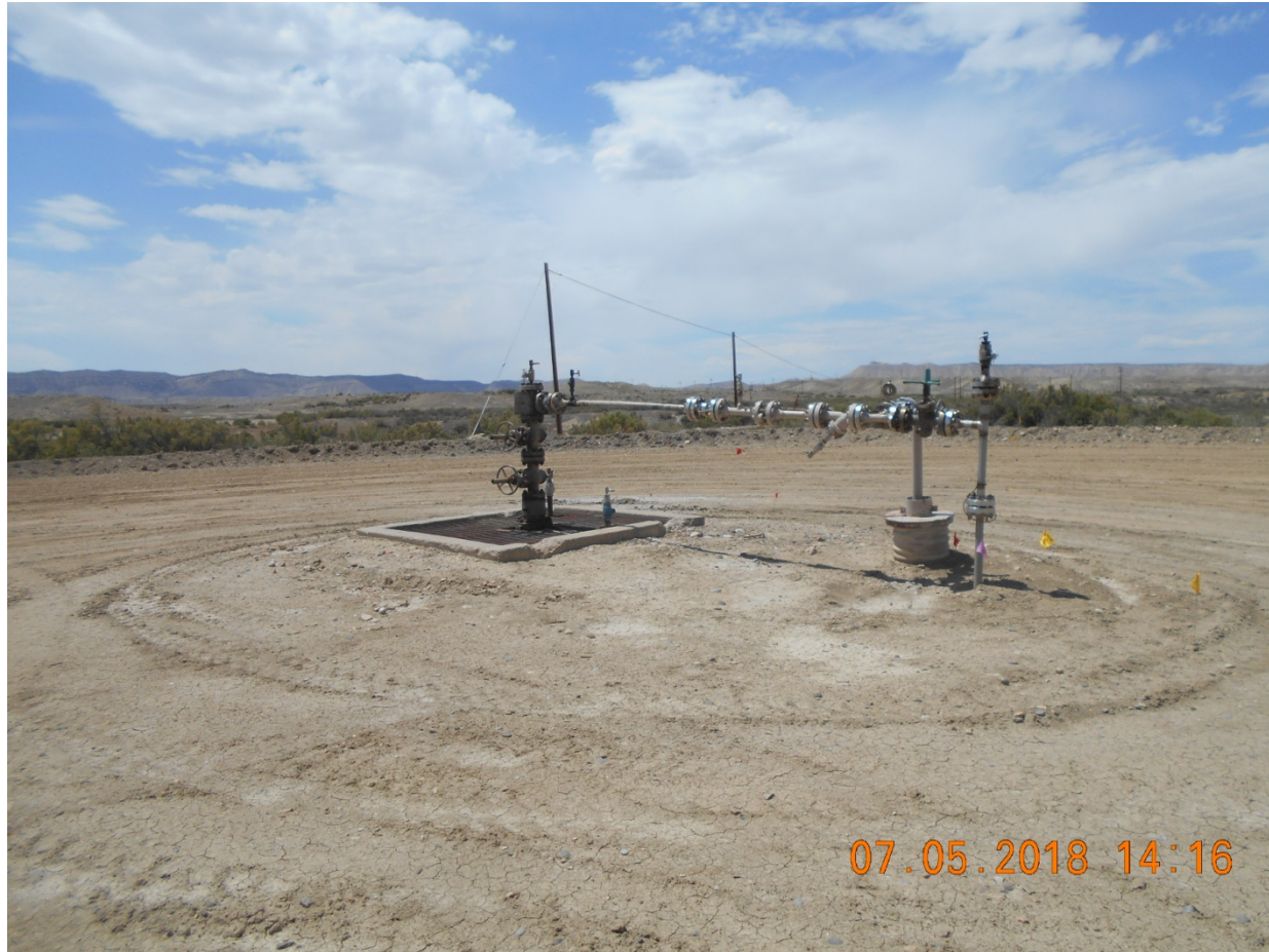
Injection Wellhead
