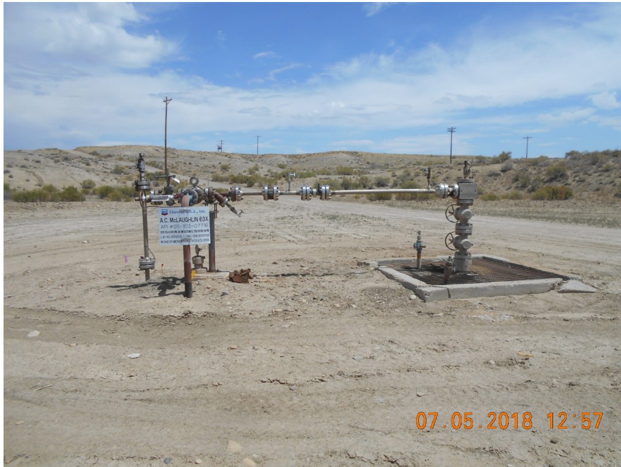
Injection Wellhead
