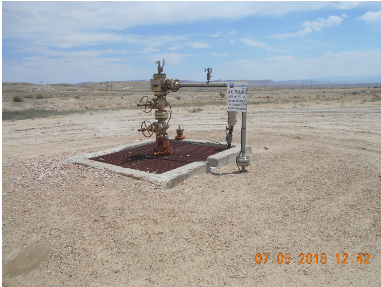
Injection Wellhead
