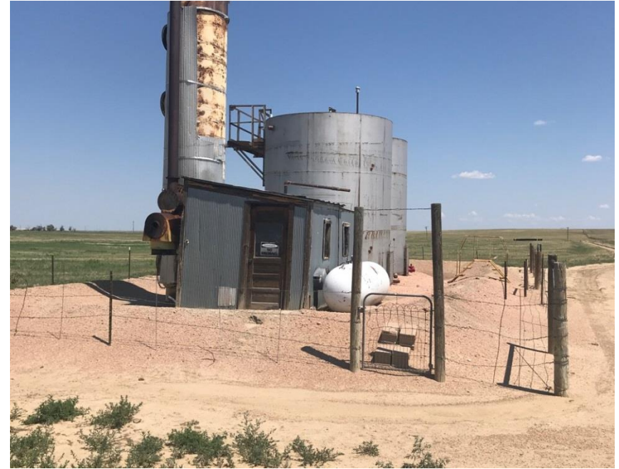
Photo#2 Vertical Heater Treater
