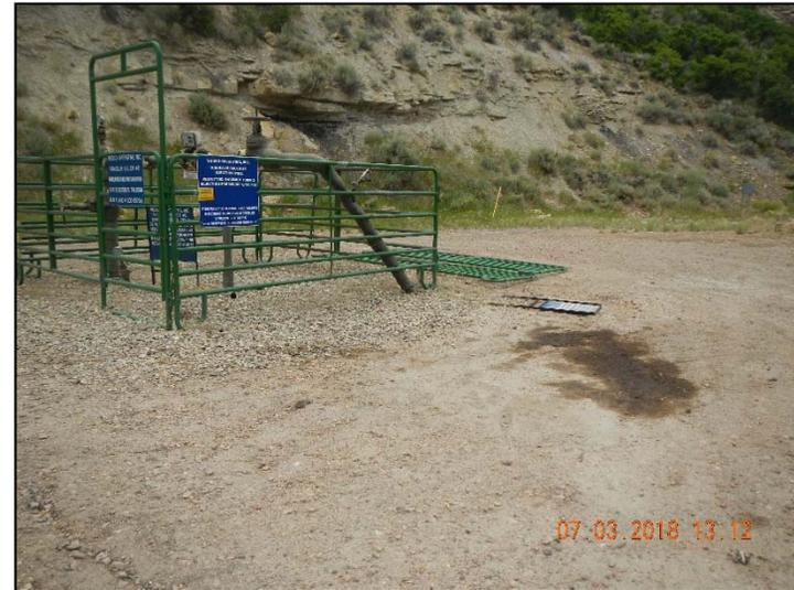
**Photo 2. Stained soil at wellhead.**
