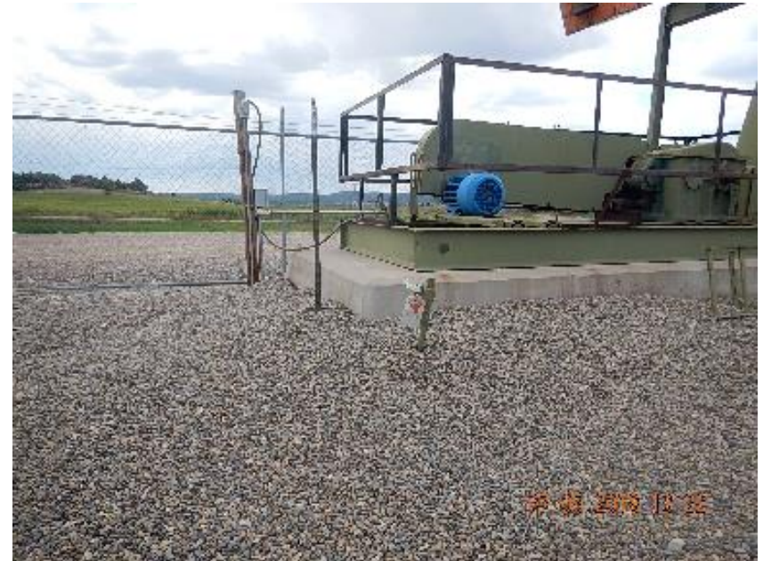
Photo 2: Unused riser at #5-1 wellhead.
