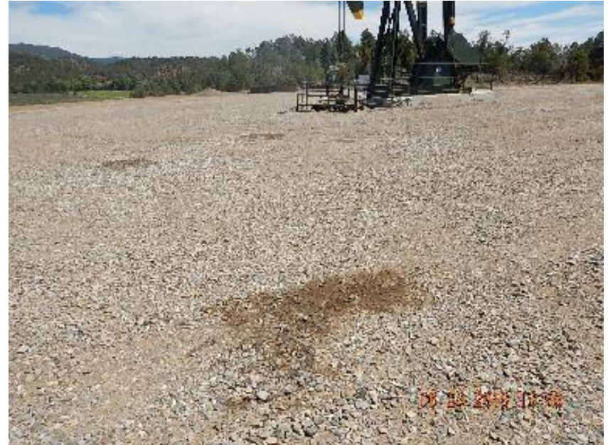
Photo 4: Impacted soil and gravel out from wellhead.
