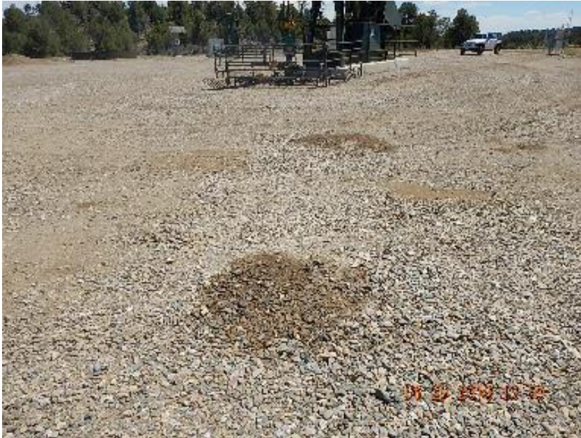
Photo 5: Impacted soil and gravel out from wellhead.
