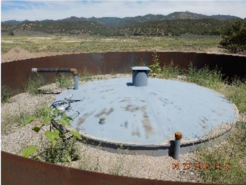
Photo 3: Production tank with no signage and vegetation growing inside containment.
