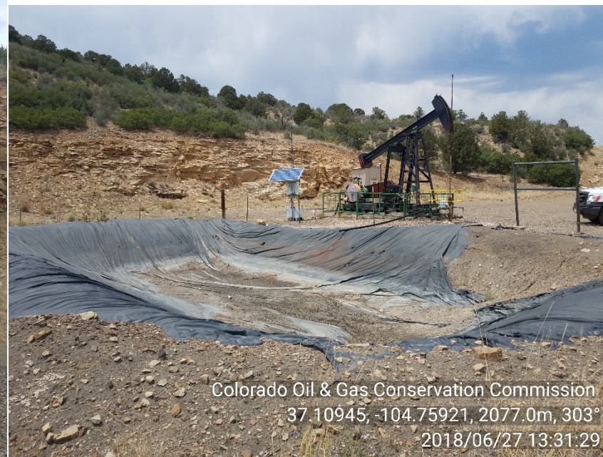
Location Photo and pit liner damage and equipment
