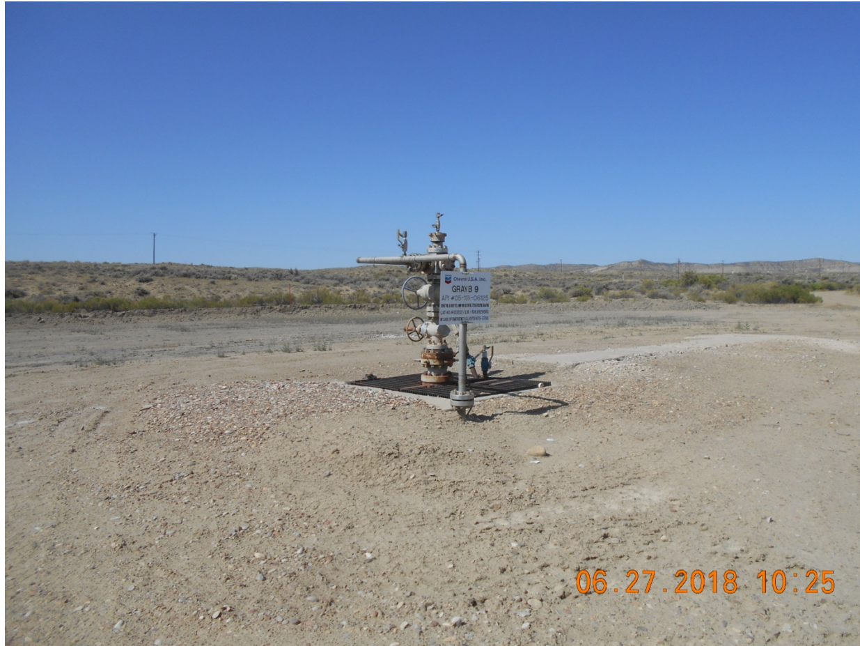
Injection wellhead.
