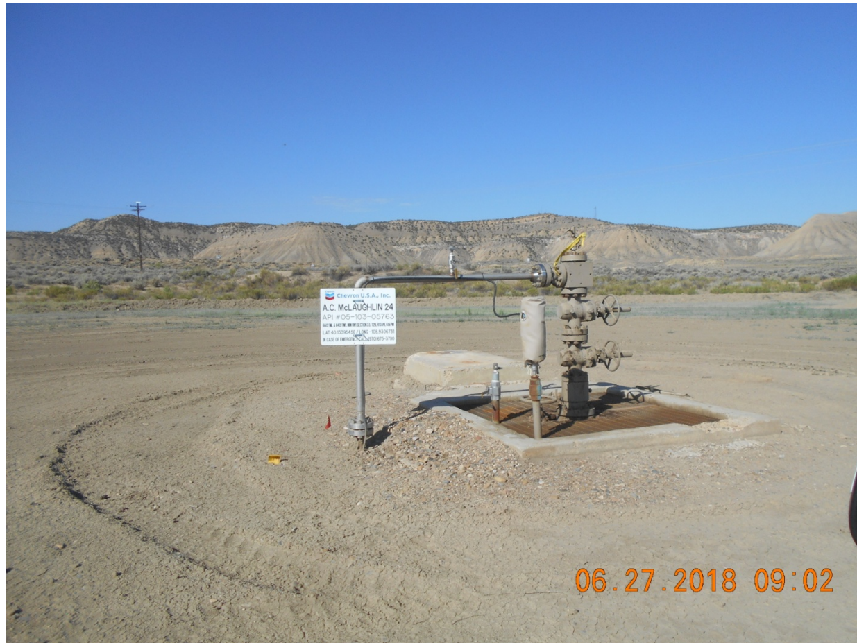
Injection Wellhead
