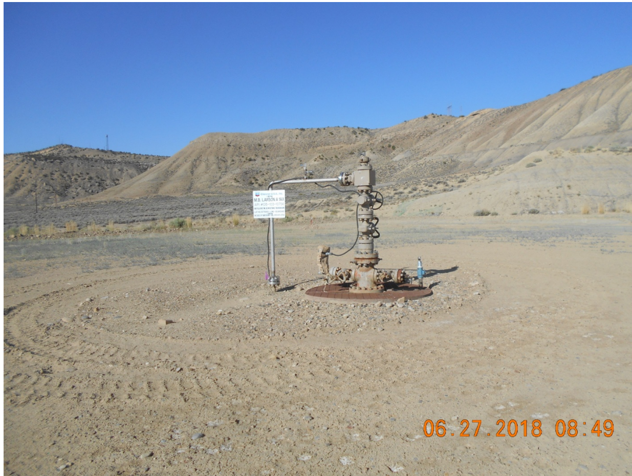
Injection Wellhead
