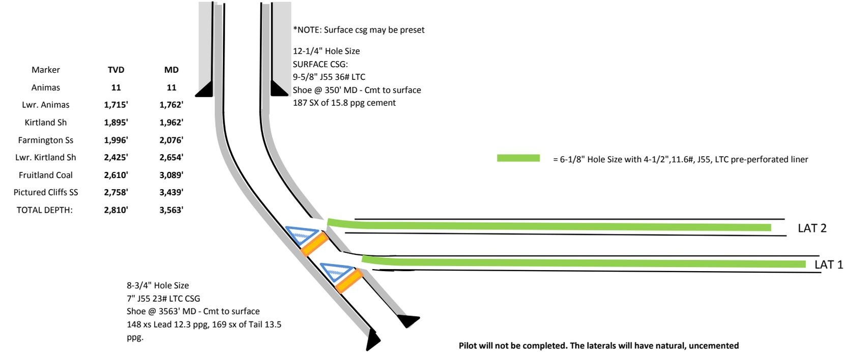
Pilot will not be completed. The laterals will have natural, uncemented completion. Liners will be run in laterals to prevent wellbore collapse.
