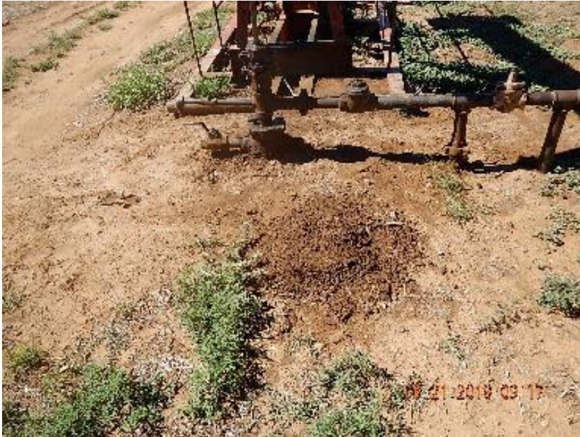
Photo 3: Impacted soil at wellhead.
