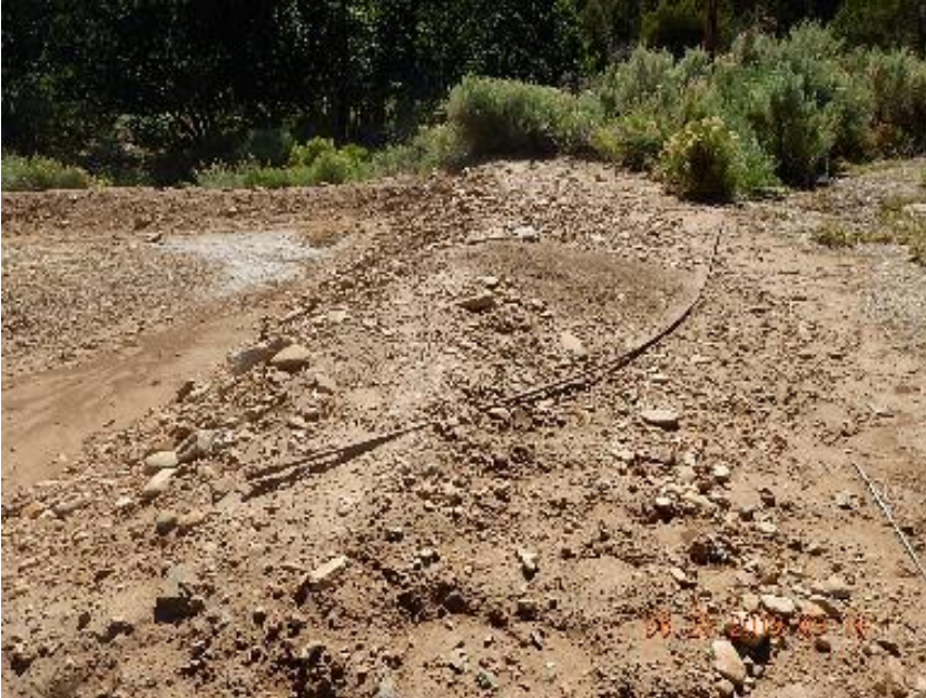
Photo 5: Bent sucker rod at tank berm.
