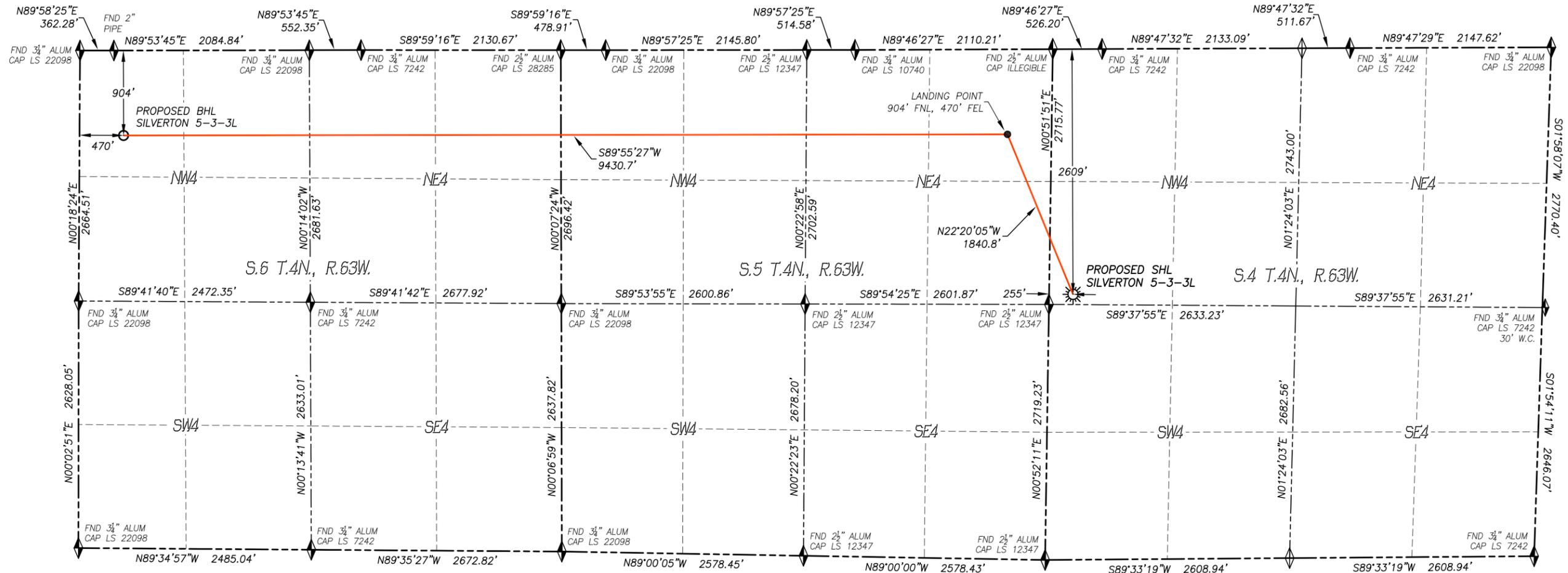
IN ACCORDANCE WITH A REQUEST FROM CONFLUENCE RESOURCES, DALEY LAND SURVEYING, INC. HAS DETERMINED THE SURFACE LOCATION OF THE SILVERTON 5-3-3L WELL TO BE 2609' FNL, 255' FWL, AS MEASURED AT NINETY (90) DEGREES FROM THE SECTION LINES OF SECTION 4, TOWNSHIP 4 NORTH, RANGE 63 WEST, AND THE BOTTOM HOLE LOCATION TO BE 904' FNL, 470' FWL, AS MEASURED AT NINETY (90) DEGREES FROM THE SECTION LINES OF SECTION 6, TOWNSHIP 4 NORTH, RANGE 63 WEST, OF THE 6TH PRINCIPAL MERIDIAN, WELD COUNTY, COLORADO.
