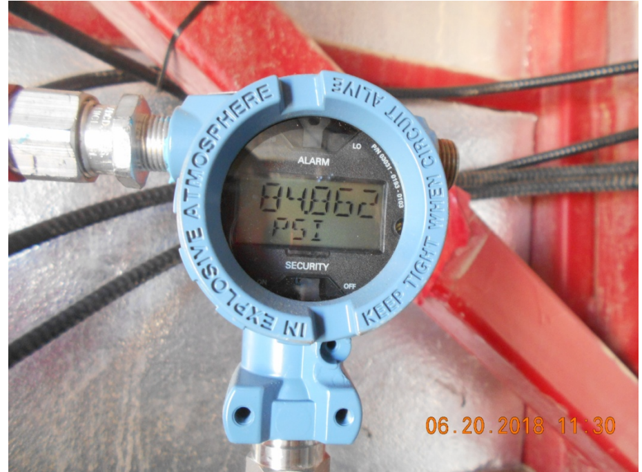
Injection wellhead tubing gauge
