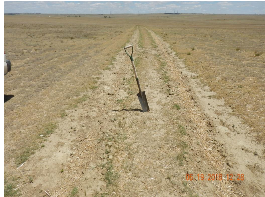
Photo 2: Photo taken from the access road, facing northeast. Photo shows inspector tested the access road for compaction concerns. Photo shows soils OUTSIDE the areas of the ruts, where a ripper DID NOT pass through, were difficult to penetrate; inspector was only able to easily penetrate the top couple inches of soil. Compaction concerns remain evident.
