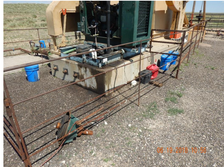
Photo 10: Photo taken from the southeast corner of the pump jack facing northwest. Photo shows numerous 5 gallon buckets with chemical and oil jugs found around the pump jack. Buckets need to be properly removed and disposed of, or placed into containment. Photo also shows unused equipment that needs to be removed.
