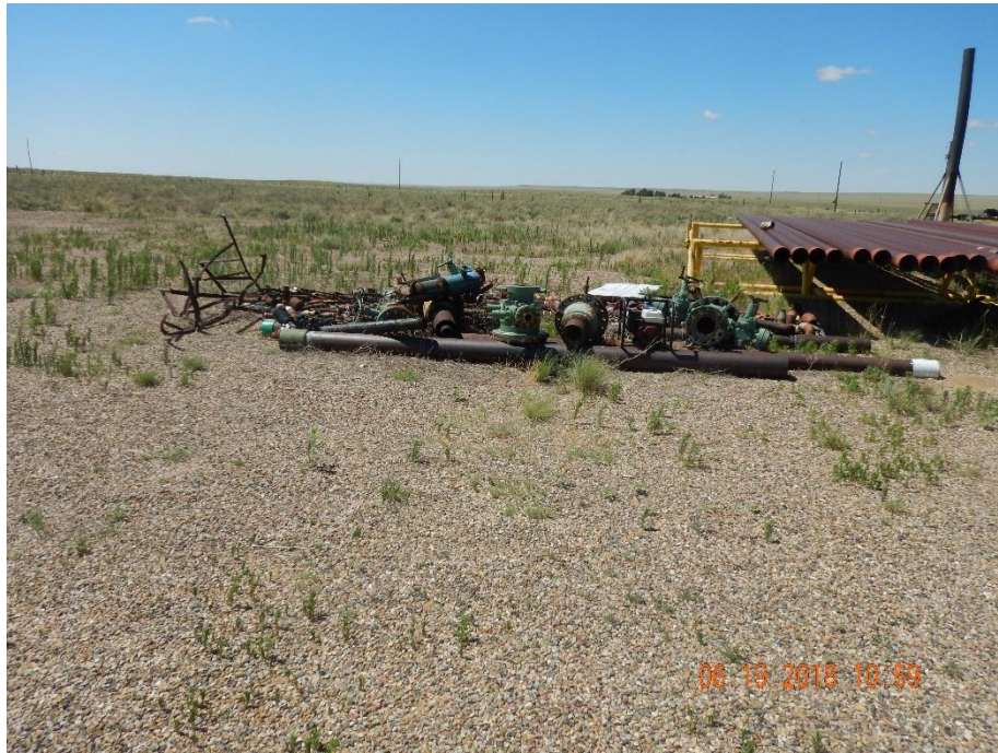
Photo 19: Photo taken from the east end of the location, facing south. Photo shows various unused equipment not needed for production being stored on location. This needs to be removed. Additionally, these areas do not appear to be reasonably needed for production and needs to be reclaimed.
