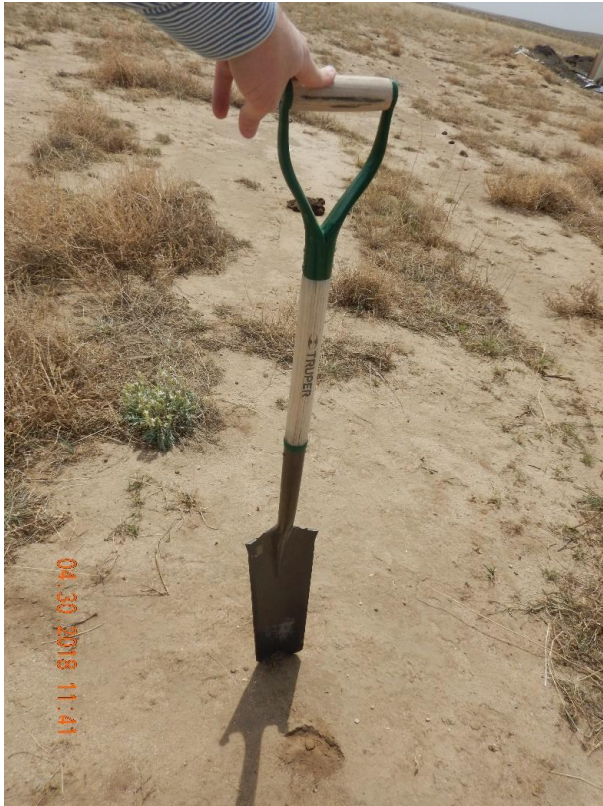
Photo 33: Photo taken from the northern interim area. There are large areas within the interim that remain predominantly bare and exposed soil. Photo shows compaction concerns appear evident within these areas as inspector had difficulty penetrating to top layer of soil with a shovel.
