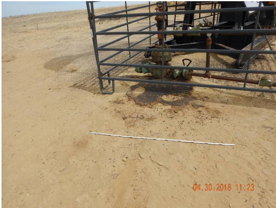
Photo 21: Photo taken from the southwest end of the well, facing north. Previous inspections required operator to remove and/or remediate oil stained soil at well head. Photo shows oil stained soil has not been removed/remediated. .
