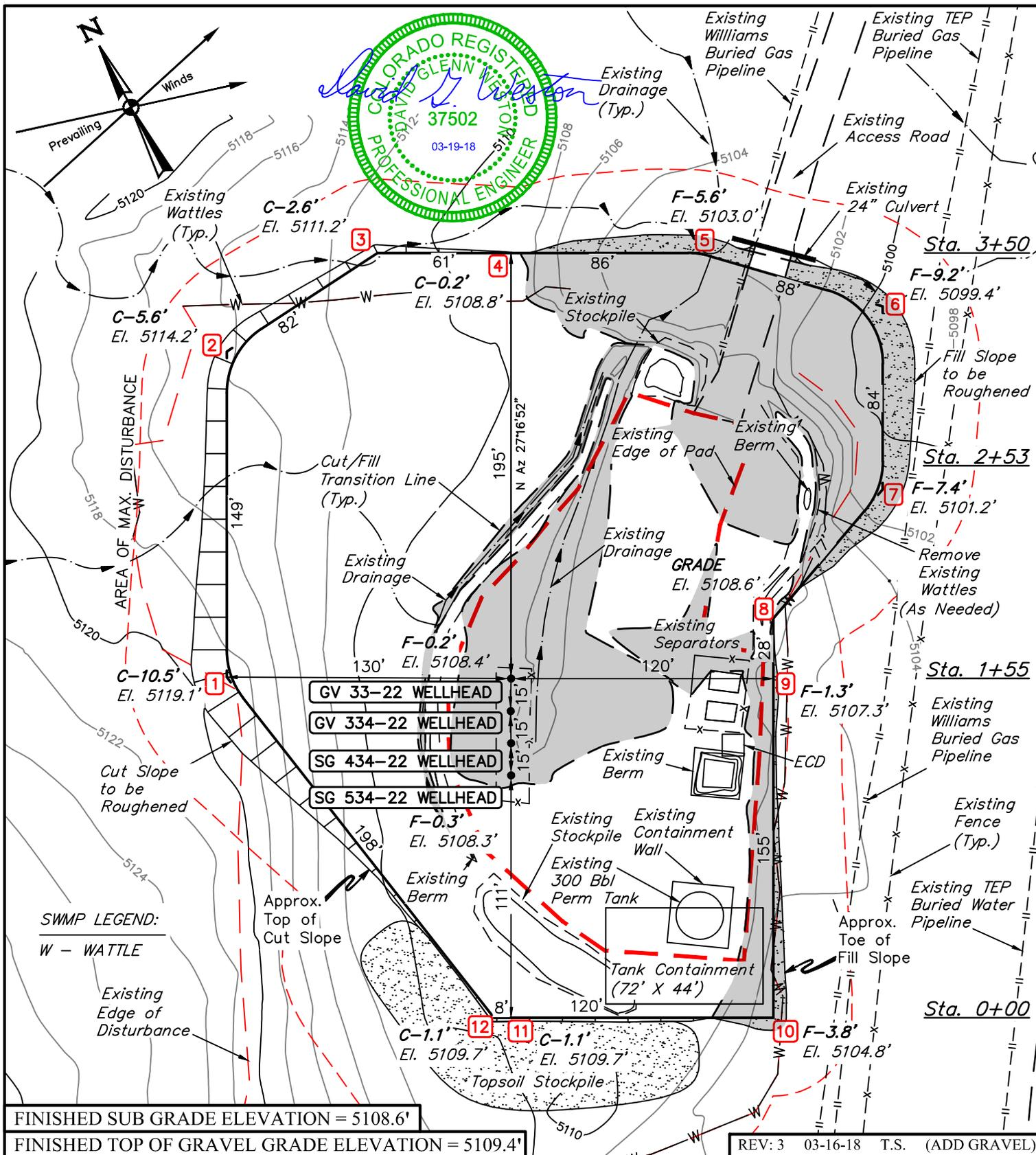
NOTE: All fill is to be compacted to a minimum of 95% of the maximum dry density obtained by AASHTO method t-99.
