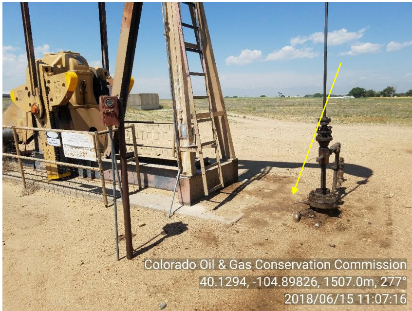
Photo 1. Wellhead/ Stained soil
