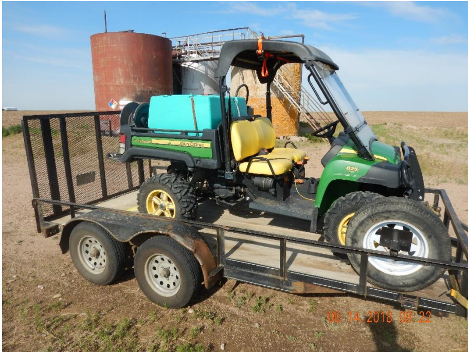
Photo 1: Photo of Gator UTV with spraying tank and booms used to apply the herbicide on location
