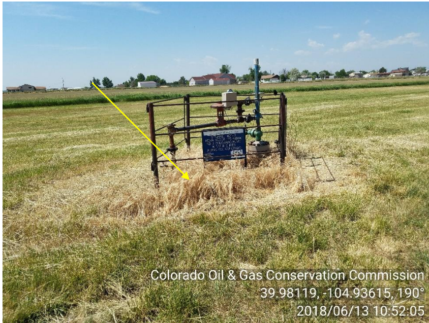
Photo 1. Wellhead, overgrown weeds/grass
