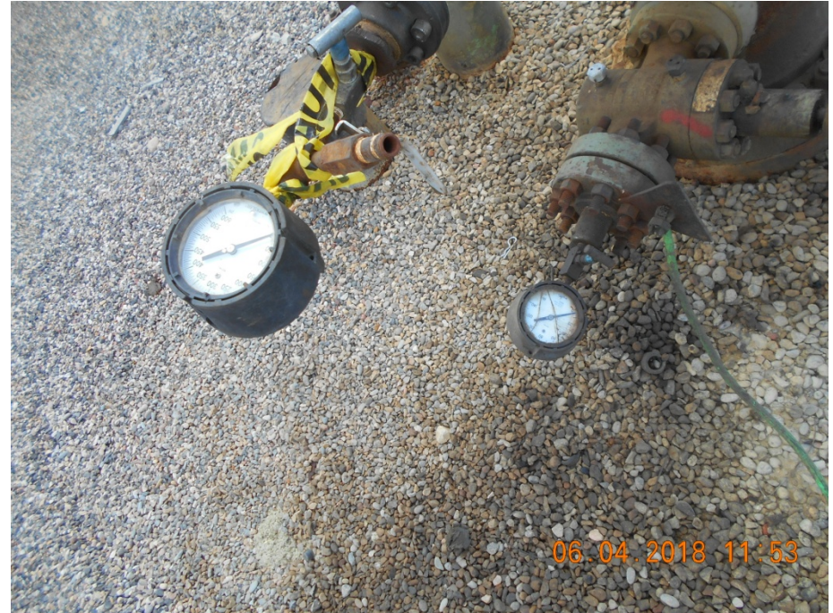
Casing and Bradenhead gauges
