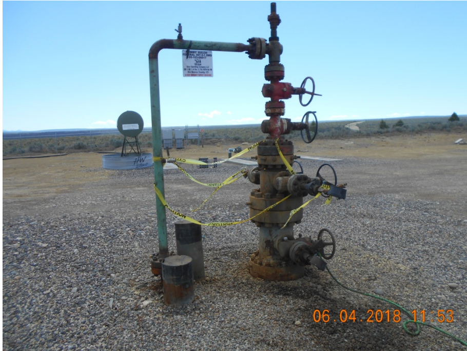
Injection wellhead
