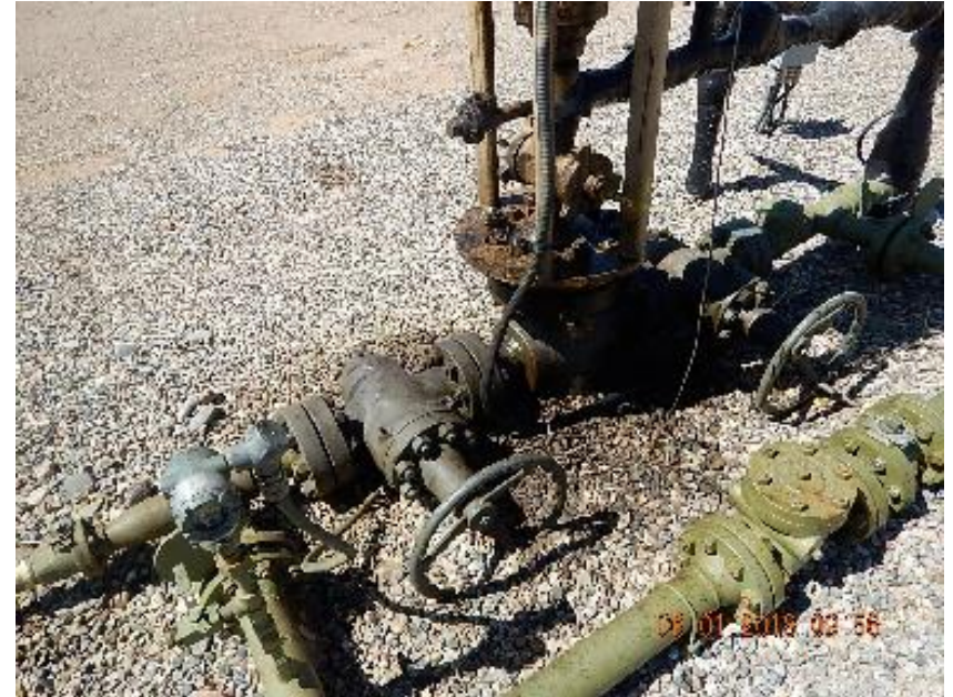
Photo 2: Impacted soil and gravel around wellhead.
