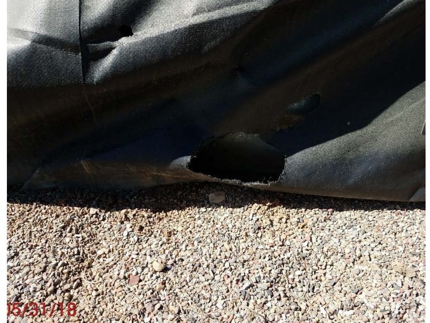
Location Photo #6, holes in battery liner
