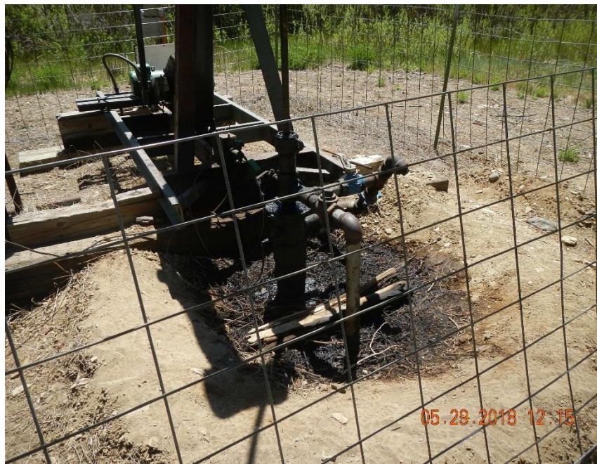
Stained soil around well head, noted in previous inspection report.
