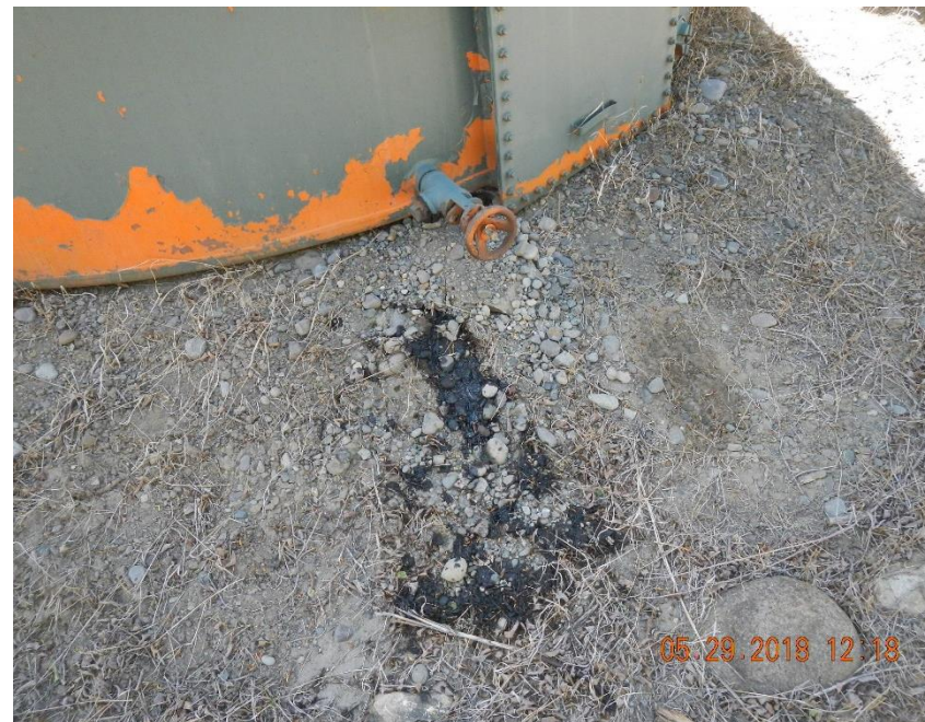
Stained soil beneath valve on AST.
