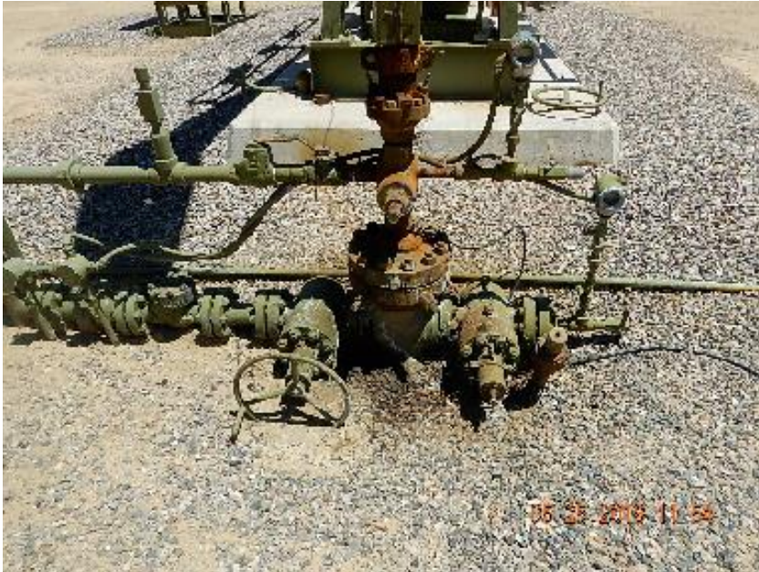
Photo 3: Impacted soil and gravel around base of wellhead.
