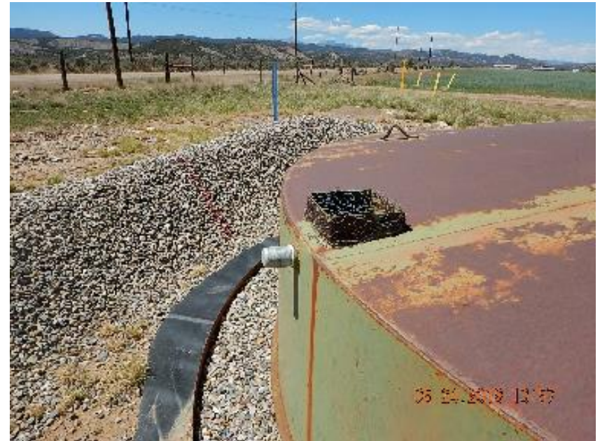
Photo 2: Covered tank opening.
