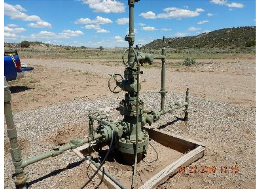
Photo 2: Wellhead set up.
